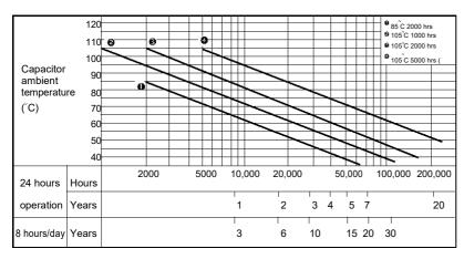
Example: When a 2000 hours/105°C guaranteed product is used continuously at 60°C, it can be expected to have a life of 5 years.
